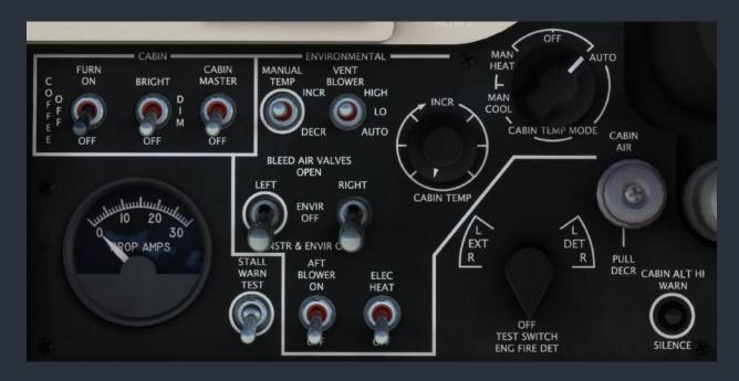
Be aware that these ventilation systems increase the load required from the current power source substantially, and therefore should be used predominantly while under power, or when external power is supplied to the aircraft. Additionally, the more bleed air that is removed from the operating engines, the more ITT will be increased. Engine performance should be increased as much as possible by reducing load for high performance takeoffs.
