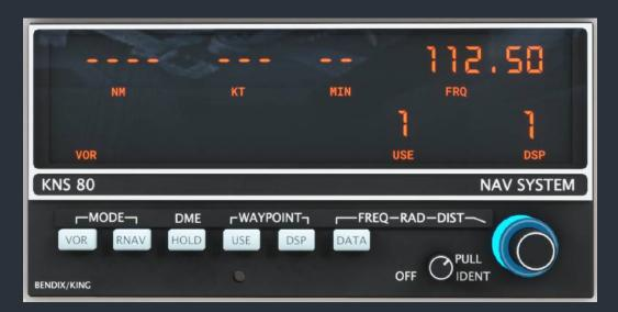
3. Once our desired frequency has been set we will use the "DATA" push button to page through the three required pieces of data in this data channel in the order "FREQ-RAD-DST". Press the "DATA" button once, and then enter the radial 154.0, again with the dual concentric rotary knobs. Should your desired radial include a decimal component, the inner rotary knob can be pulled and rotated for decimal entry.
