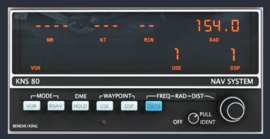
4. When our desired radial is set, press the "DATA" push button once again to enter our desired distance offset of 12.3 nm. Again, should your desired distance include a decimal component, the inner rotary knob can be pulled and rotated for decimal entry.
